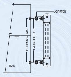
The gauge is side mounted to the tank through thread fittings, ensuring that it is mounted in plumb. CC distance between tank fittings should corresponds to CC dist. of gauge, failing which it may cause gauge glass damage / breakage.
